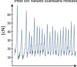
Typical release values on PET film. Direct comparison using 180°C at 1000 mm/min to peel off the liner from the Butyl. 24h storage at 40°C under 2 kg weight.
