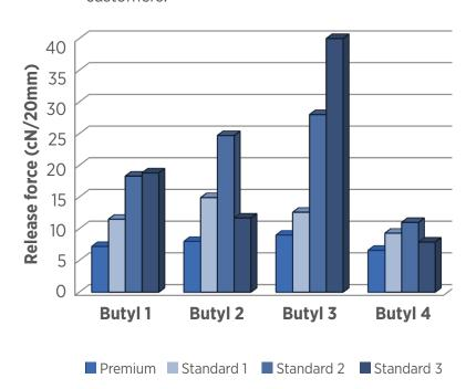
24h storage at 40°C under 2 kg weight, cooling down for 1 hour at room temperature.
